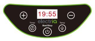
increments. Press the "TIMER" button to set the timer. The timer is selectable with 30 minute increments up to 48 hours. After the timer lapsing fan will continue to run for approximatively 10 more seconds than will go in standby.
