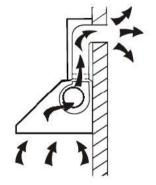
An adaptor is also supplied to enable you to connect your hood to pre-existing 120mm diameter ducting.
