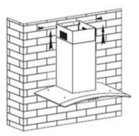
Place the two chimneys together onto the cooker hood body. Adjust the height of the inner chimney until a suitable height. Fix the inner chimney to the chimney bracket using the supplied screws (ST4\*8).
