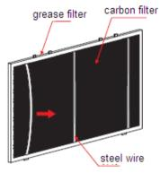
2. Unclip the wire from the reverse of the grease filter.
