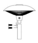
**Step 4:** Place the heater head gently onto the stem and secure it with the 2 bolts provided. Then secure the power cord to the base using the cable clip. Your heater is now ready to use.
