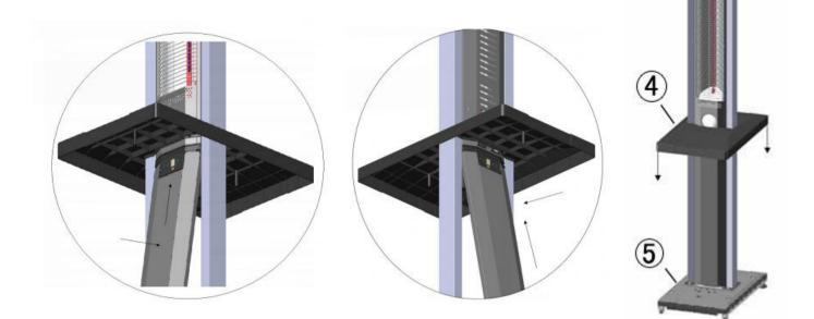
**STEP 6:** Secure the base into place using two WASHERS (7) and two ST3.5×12 Screws (8).
