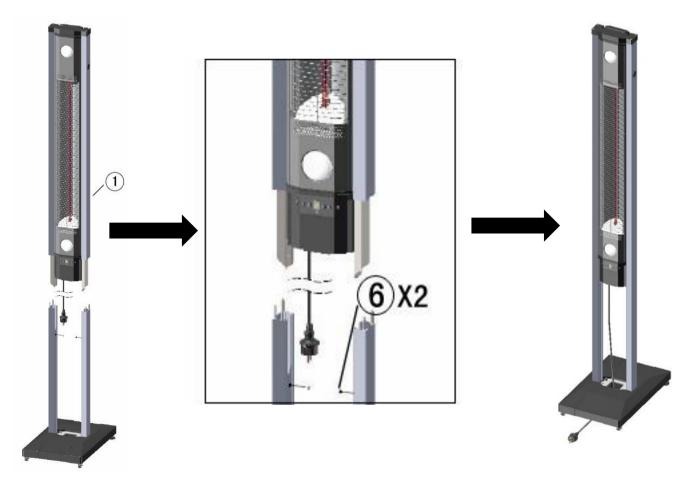
**STEP 5:** Slide the BASE COVER (4) up to the base of the main body, gently push both PANELS (2) into position until they are securely in place. Do not complete this step until you have successfully pulled the power cable through the base. When complete, slide the BASE COVER back down so it is back in its original place.
