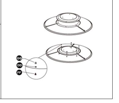
Attach the Reflector Assembly to the Head Assembly (C). Secure with cap nuts (GG) and  $\Phi$ 6 washers (DD).
