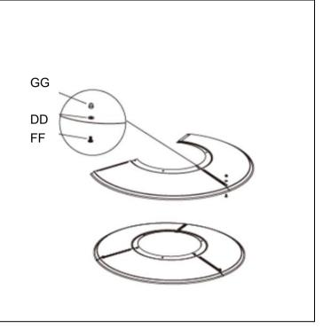
Attach the Reflector Plate (B) to the Reflector Panels (A) using M6 x 8mm Screws (FF), Φ6 washers (DD) and Cap Nuts (GG). Do not fully tighten at this point.
