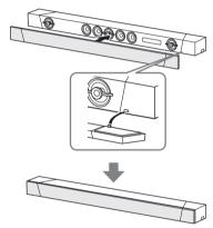
**Tip**The grille frame is fixed by a magnet.
