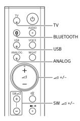
Press TV, ANALOG, BLUETOOTH, or USB to select the input that the desired device is connected.
