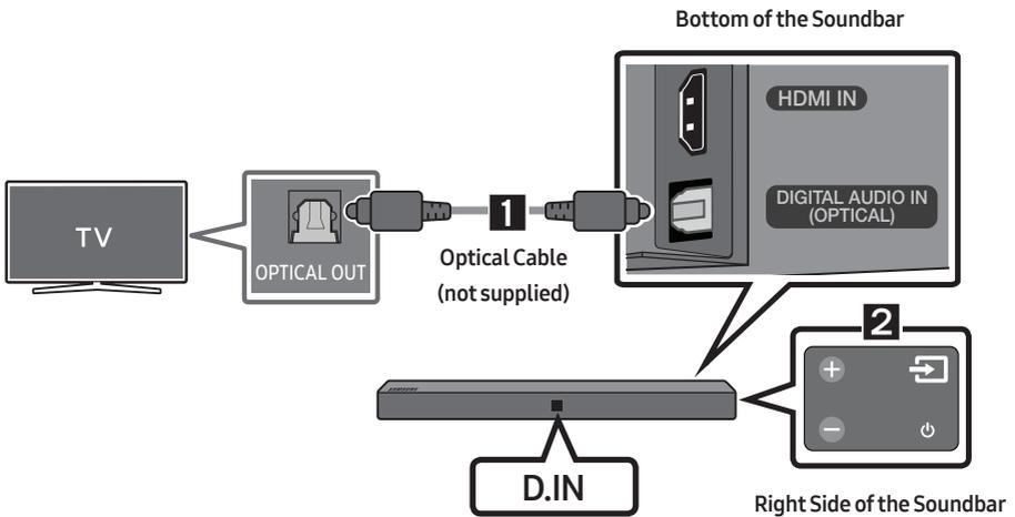
1. Connect the **DIGITAL AUDIO IN (OPTICAL)** jack on the Soundbar to the **OPTICAL OUT** jack of the TV with a digital optical cable (not supplied).
