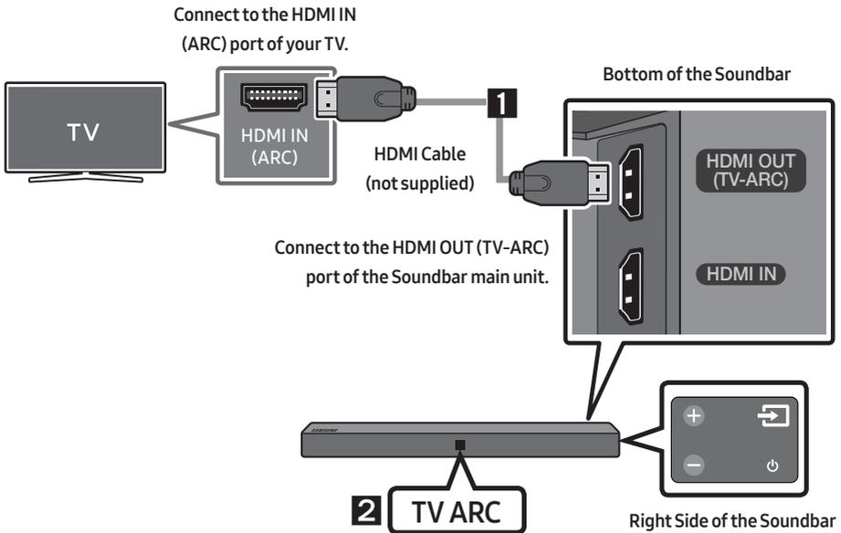
1. With the Soundbar and TV turned on, connect the HDMI cable (not supplied) as shown in the figure.
