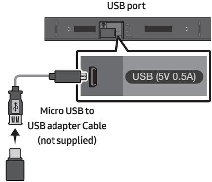
If an update is offered, you can update the firmware by connecting a USB device with the firmware update stored on it to the USB port on your Soundbar.
