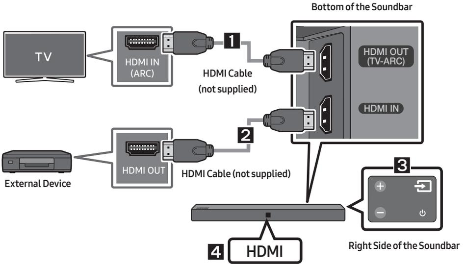
1. Connect an HDMI cable (not supplied) from the **HDMI OUT (TV-ARC)** jack on the back of the product to the HDMI IN jack on your TV.
