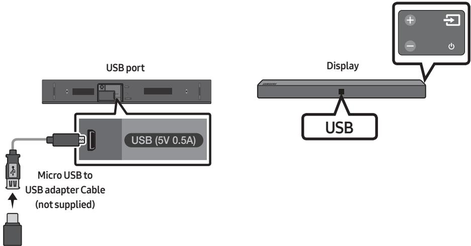
1. Connect a Micro USB to USB adapter cable with a male USB 2.0 Micro USB plug (Type B) on one end and a standard female 2.0 USB jack (Type A) on the other to the micro USB jack on your Soundbar.
