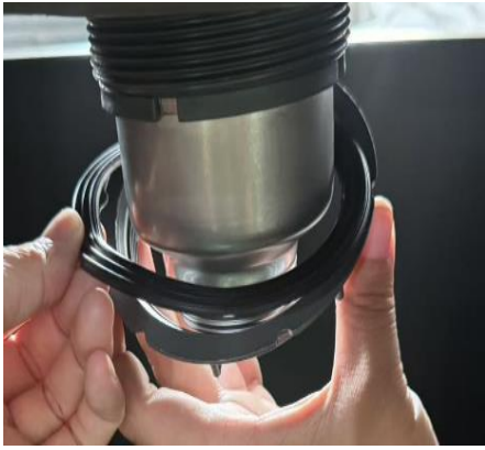
Insert the funnel bottom seal(3) followed by funnel bottom ring(6). Rotate ring to tighten.
