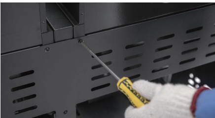
43 Fix the Rear Body Panel (30) using seven Bolts (A).
