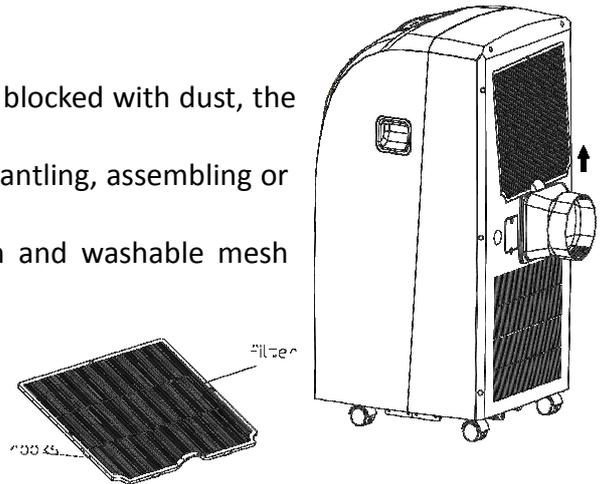
**Please note:** If in use, the optional active carbon filter (cloth) should be replaced every 3-6 months based on the environment.
