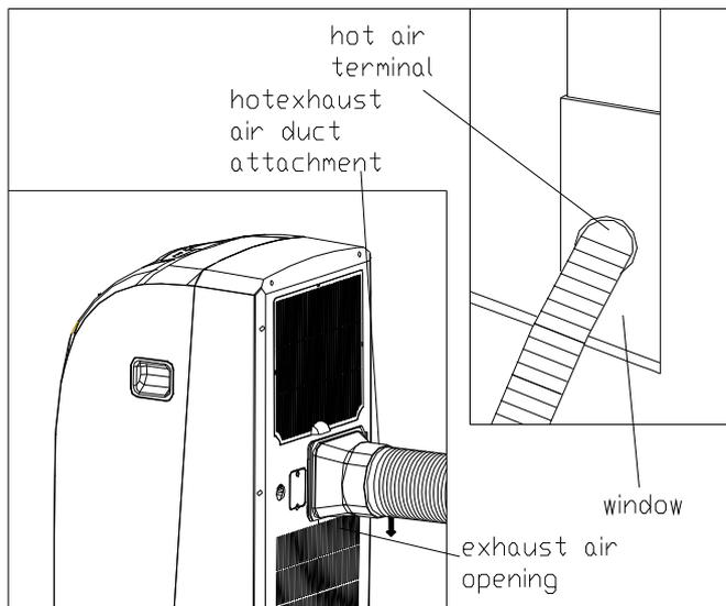
3. Extend one head of the hose and screw it into the assembled adaptor at the back of the unit anti-clockwise.
