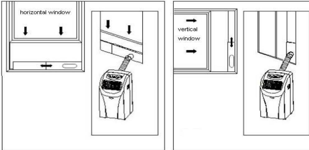
**Note:** The window kit is only designed to be installed with sliding or sash windows or doors. The window kit is not designed or to be used with any other style of windows. However the fish tail adaptor can be used with most windows / doors.
