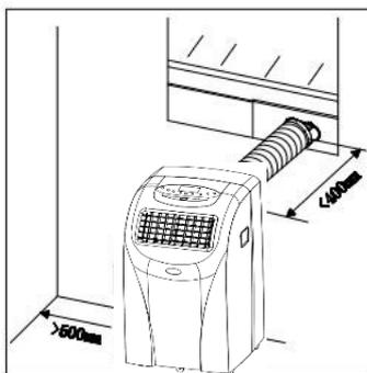
The length of the soft hose extends from 28 cm to 150 cm. If hose is extended above this length the unit may malfunction and this can invalidate the warranty.
