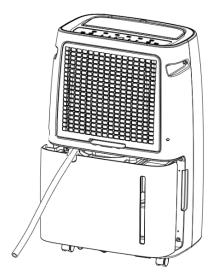
Make sure the connection between pipe and the drain outlet is tight and does not leak. Then direct the pipe to a suitable drainage point. This unit uses gravity to dispose of water hence the drain should be lower than the water outlet on the unit. Put the tank back into the unit. Be sure to run the water pipe downward and let the water to flow out smoothly. Do not kink or bend the pipe.
