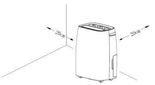
Your electriQ dehumidifier will begin to protect your space from the harmful effects of excessive moisture as soon as it is turned on. Excess moisture is dispersed throughout your home. For this reason, the dehumidifier should be positioned in a central and clear location so that it can draw this moist air towards it from all over the home. A warm hallway or landing is an excellent position for your dehumidifier. If possible, leave interior doors ajar to allow air circulation.
