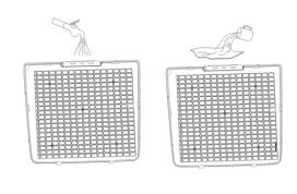
Remove the ABS filter frame. If the mesh filter is dirty, hoover it. If it is heavily soiled wash it with warm soapy water and dry thoroughly before reinserting it in the unit.
