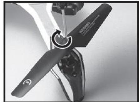
It is important for the correct blade to be placed on the correct motor or the aircraft will not fly correctly. Each blade is marked with an A or B to indicate which motor it corresponds to.
