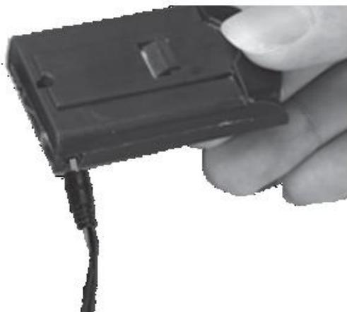
Plug the charger into the USB socket before attaching the battery.
