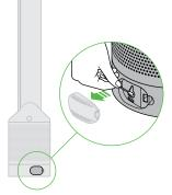
Clean the hatch every time the filter is replaced. Open the small hatch on the side of the appliance. Use a cotton bud to clean inside and remove any debris. This maintains sensor accuracy and ensures the continuing high performance of the appliance.
