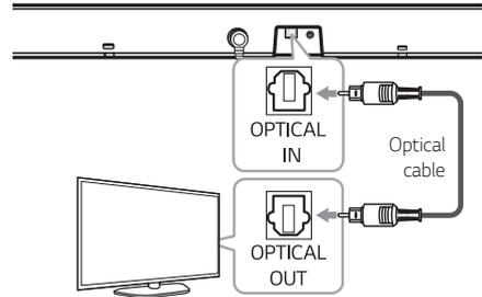
2. Select the input source to OPTICAL by pressing **F** button on the remote control or unit repeatedly.
