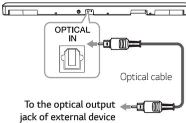
1. Connect the OPTICAL IN jack on the back of the unit to optical out jack of your external device.
