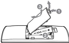
Remove the battery cover on the rear of the remote control, and insert the battery  $\oplus$  with  $\ominus$  and matched correctly.
