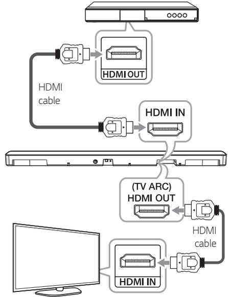
1. Connect HDMI IN jack on the back of the unit to HDMI OUT jack on the external device such as Blu-ray disc player, DVD player, etc.
