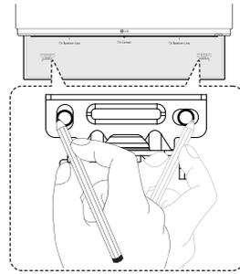
3. Remove the Wall bracket install guide.
