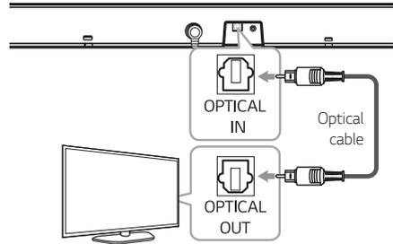
2. Set up the sound output of TV to listen to the sound through this unit :
