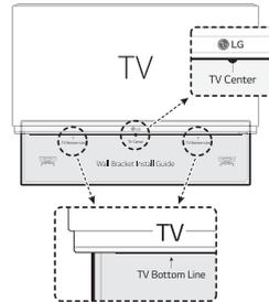
2. When you mount it on a wall (concrete), use the wall plugs. You should drill some holes. A guide sheet (Wall bracket install guide) is supplied to drill. Use the sheet to check the point to drill.
