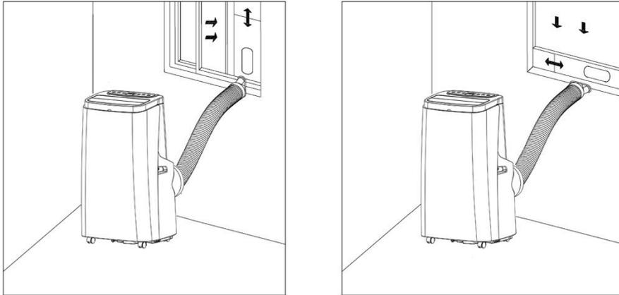
**Note:** The window kit is only designed to be installed with sliding or sash windows or doors. The window kit is not designed or to be used with any other style of windows. However, the fish tail adaptor can be used with most windows / doors. When using the cooling mode ensure that the opening left is as small as possible. The best form of installation is through a wall duct. By properly venting, you expel hot air from your room while efficiently cooling it.
