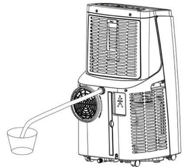
**Note:** This model has a self-evaporative function, which reduces the need to empty the water tank. If the unit is vented correctly most of the water is reused to cool the condenser coils and any excess is evaporated. Please do not use continuous drainage if you intend to use the self-evaporating facility.
