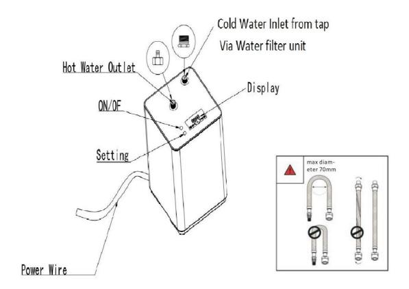
Avoid kinking tubes during installation as this could restrict flow and cause malfunctioning of appliance. Do not use pipe sealing compounds on any connections. These can foul the internal mechanics and may cause objectionable taste and odour.
