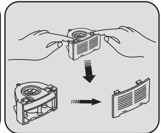
3. Turn out the fan assembly and pull the two buckles, then the fan will be opened.
