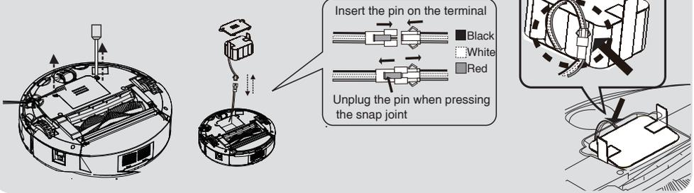
1. Loosen the screw with a screwdriver to unfold the battery cover.
