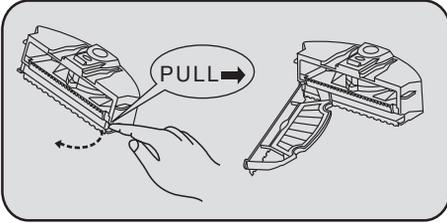
1. First, pull out the dust box, then push the buckle on the double side and open the panel.
