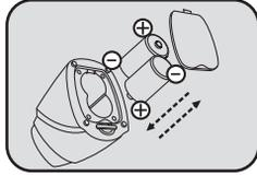
2. Put 2 D alkaline batteries into the battery slot, making sure to match the positive and negative signs on the battery to the correct end of the battery slot.
