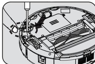
3. Put the side brush back in its hole, and put the screw back in the side with a screwdriver.
