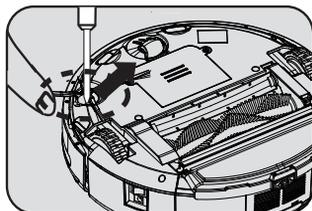
1. Take out the screw on the side brush with a screwdriver.
