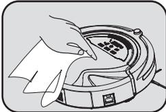
1. Before cleaning the main body, please turn off the power switch and take out the power plug.
