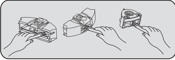
Pour out the dust, then use a clean brush to clean the dust box and fan assembly. Take out the fan assembly and then clean the dust box.
