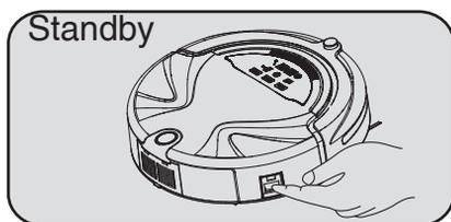
1. Press AUTO on the vacuum or the power button on the remote control. The display will light up, meaning that the robot is on standby.
