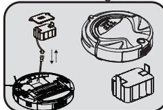
If the machine is not used for a long time, please fully charge the battery, take it out and put it in a cool dry place, keeping the bottom of cleaner dry.
