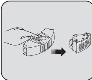
2. Press the red button on dust box and the fan assembly will automatically pop up.
