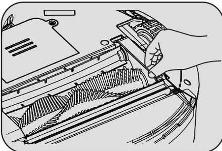
1. As shown on the above photo, push the buckle and lift it up.
