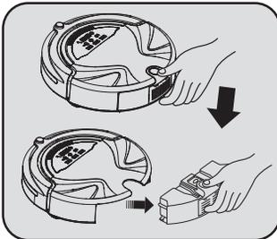
1. Push the buckle on the double side, then take off the front panel.
