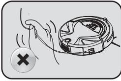
⚠ Do not pull the machine by the power cord. Do not twist or bend the wire or put anything heavy on it.
