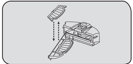
4. Push the old filter out from the buckle and then replace with a new and clean one .
