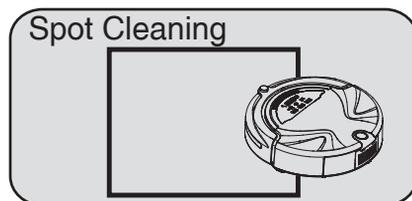
3. When you press the SPOT button, the robot will start to work under spot mode. To stop the cleaning, press any button on the vacuum.
