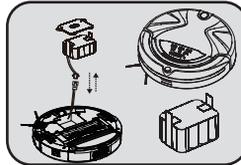
If you haven't used the vacuum for a long time, fully charge the battery, take it out, and keep it in a cool, dry place, keeping the bottom of the cleaner dry.
