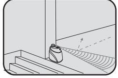
4. Put the zone divider on a flat bit of floor and against a wall as a barricade from where you want to stop the vacuum from going.
