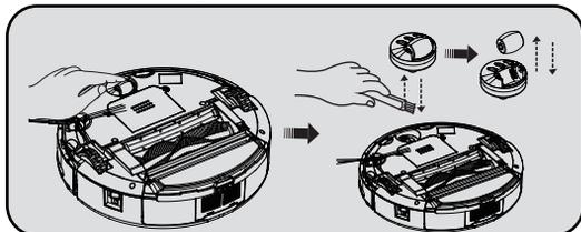
1. Pull out the front wheel with fingers or a tool. (as picture)
