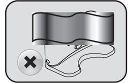
3. Do not cover the signal window of the charging station, otherwise the auto-charging function won't work.
