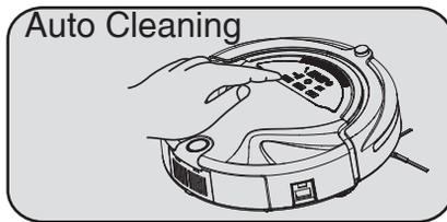
2. Press the AUTO button again and the robot will start to clean automatically. To stop the cleaning, press any button on the vacuum.
