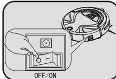
If you're not using the machine, please turn off the power or else it will damage the battery.
