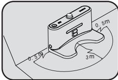
1. Put the charging station on a flat floor and against the wall, to make sure the vacuum can get back to the station. Ensure there are no obstacles or drops in the floor for 3 metres in front and 0.5 metres on the left and right of the charging station.
