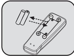
2. Put 2 AAA alkaline batteries into the battery slot, making sure to match the positive and negative signs on the battery to the correct end of the battery slot.
