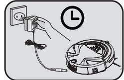
The battery should be charged for 12 hours if it hasn't be used for a long time or for the first time. Use the cleaner for up to 3-4 charges for the best battery efficiency.
