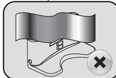
Do not cover the signal window of the charging station or else the function of auto-charging won't work properly.
