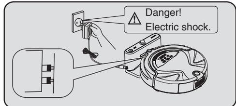
2. Connect the plug between the adaptor and charging station. Then, put the electrodes on the vacuum against the electrodes on the charging station. Finally, connect the power socket.
