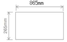
865 x 265 mm. Make sure that the edges of the hole are at least 35mm from the edges of the cupboard.
