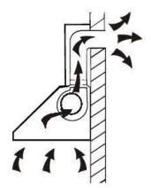
A 150mm diameter flexible pipe is provided which allows the cooking odours to be extracted outside. If this is the chosen installation method a suitable vent pipe should be purchased (150mm diameter) and consideration to the route of the vent pipe should be made. The unit is also provided with an adaptor allowing pre-existing 120mm ducting to be used to vent the unit.
