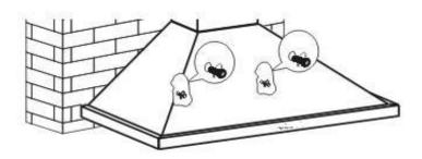
5. Remove the grease filter and fix the appliance using 2 screws (4mm x 30mm).  Plate I and II are used to fix the chimney onto the wall. Put the inner chimney into the outer chimney. Mark the position for plate II. Then pull the inner chimney upwards to the desired height, and mark the position of plate I.
