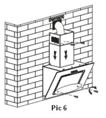
6. Fix the cooker hood with 2 ST4\*30mm safety screws. Note: The two safety vents are positioned on the back housing, with diameter of 6mm. Put the two chimneys onto the cooker hood, fix the outside chimney on the wall with 2 ST4\*40mm screws and lead the expansion pipe to the outside. See pic 6.
