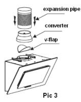
4. Install the v-flap and converter onto the cooker hood. Fix the expansion pipe on the converter using a cable tie. See Pic 3. Hang the cooker hood onto the hook.
