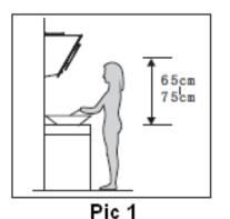
2. The cooker hood should be placed at a distance of 65~75cm above the cooking surface for best effect.
