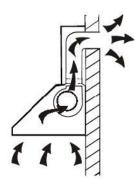
If you have an outlet to the outside, your cooker hood can be connected as below picture by means of an extraction duct (enamel, aluminum, flexible pipe or non-flammable material with an interior diameter of 120/150mm)
