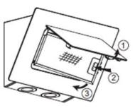
Activated carbon filter can be used to trap odors. Normally the activated carbon filter should be changed at three or six months according to your cooking habits. The installation procedure of activated carbon filter is as below.
