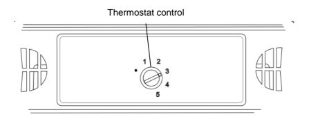
The temperature control dial can be found on the bottom of the unit. The dial can be adjusted between 1 and 5.
