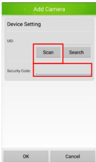
3. Use the scan button to scan the QR code on the under side of the camera, or alternatively the code from the bottom of the QR code label can be typed into the UID Box. The default password of 'admin' should also be entered in the Security Code box. Press the OK button in the bottom right.
