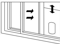
This method works with sash or vertical sliding windows. The window adapter can be placed both horizontally or vertically. It can be also installed using the trough the wall mounting adapter.
