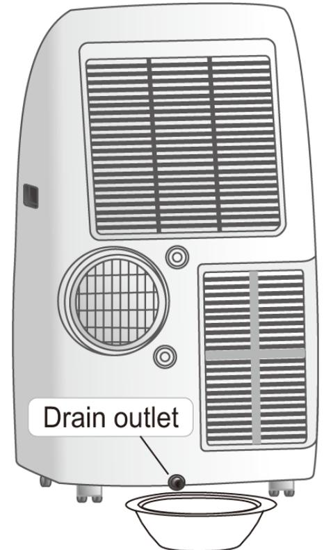
**Note:** This model has a self-evaporative function, which reduces the need to empty the water tank.
