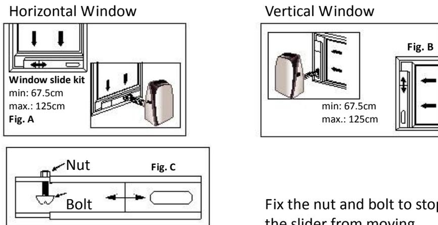
Fix the nut and bolt to stop the slider from moving.
