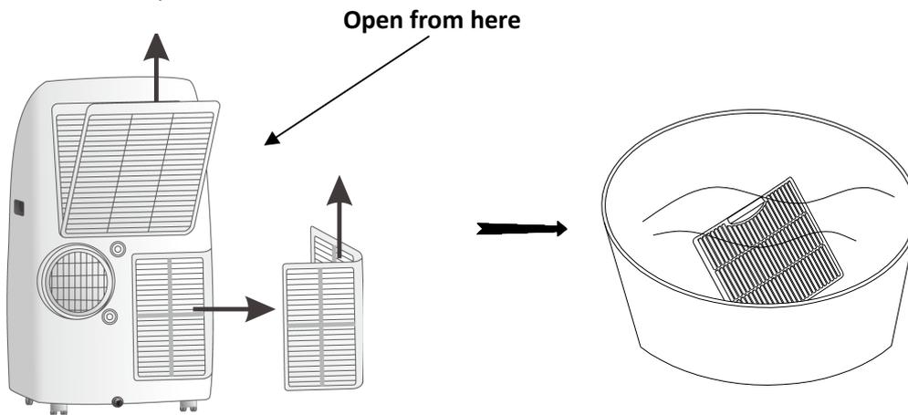
**Please note:** If the optional active carbon filter is in use it should be changed every 2-3 weeks based on the environment. The unit can be installed with HEPA filters but this may reduce its efficiency.
