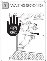
The temperature indicator (12) will go out once the thermobloc is at the correct operating temperature.
