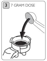
Using the measuring spoon (19), measure out one level spoon per serving into the filter. Use 2 level spoons if using the 2 cup filter.
