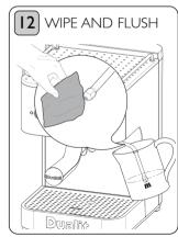
After each use, wipe the steam wand and flush the inside of the wand by dispensing water and some steam through the wand.
