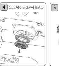
Remove the showerhead and gasket then thoroughly clean the area with a soft brush removing any coffee grounds you can see.
