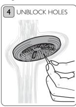
Unblock the holes of the showerhead using a pin.
