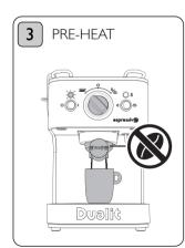
Dispense a mug full of water (min 240ml) through the machine. Ensure NO coffee is in the filter holder (5).
