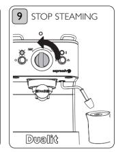
Once you have the desired amount of frothed milk, turn the control knob to the off position then move the jug away from the nozzle.
