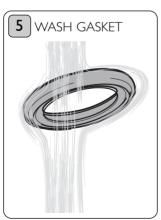
Wash the gasket with warm soapy water. Make sure there is no dried coffee or damage to the gasket. Reverse to re-assemble and test.
