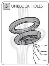
Unblock the holes of the showerhead using a pin. Wash the gasket and showerhead with warm soapy water and rinse thouroughly.
