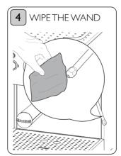
After each use, clean the wand with a damp cloth. There should be no milk residue visible.
