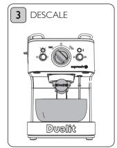
Place a large container on the drip tray. Operate as if making coffee and steaming until the tank is empty.
