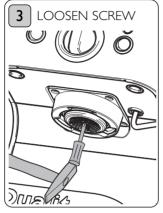
Using a screwdriver (pozi no 2) and hammer, **gently** tap the screw to dislodge any dried coffee. Then unscrew anti-clockwise.
