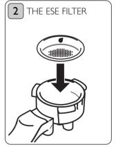
Select the ESE pod filter (16) and snap into the filter holder (5).
