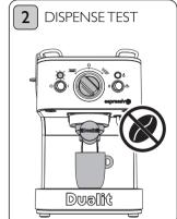
Dispense water through the brewhead (4). Ensure NO coffee is in the filter. If you see water go to fig 3. If not, turn off immediately and see fig 4.
