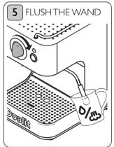
After steaming milk, flush the inside of the wand by passing water and some steam through the wand.
