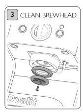
Remove the showerhead and gasket then thoroughly clean the area with a soft brush removing any coffee grounds you can see.
