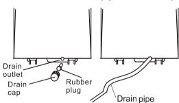
fitted as shown: use a piece of 18mm diameter tube (not supplied) and run the pipe to a drain, making sure that it runs downhill all the way.
