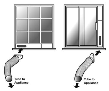
Keep the hose as straight as possible, avoid dips where the moisture from the exhaust air can condense and fill the tube with water. Do not allow the hose to be crushed.
